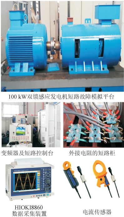
图 5 100 kW 双馈感应发电机匝间短路故障实验台及部分设备 Fig.5 Inter-turn short-circuit fault test bench and partial equipment for 100 kW DFIG
